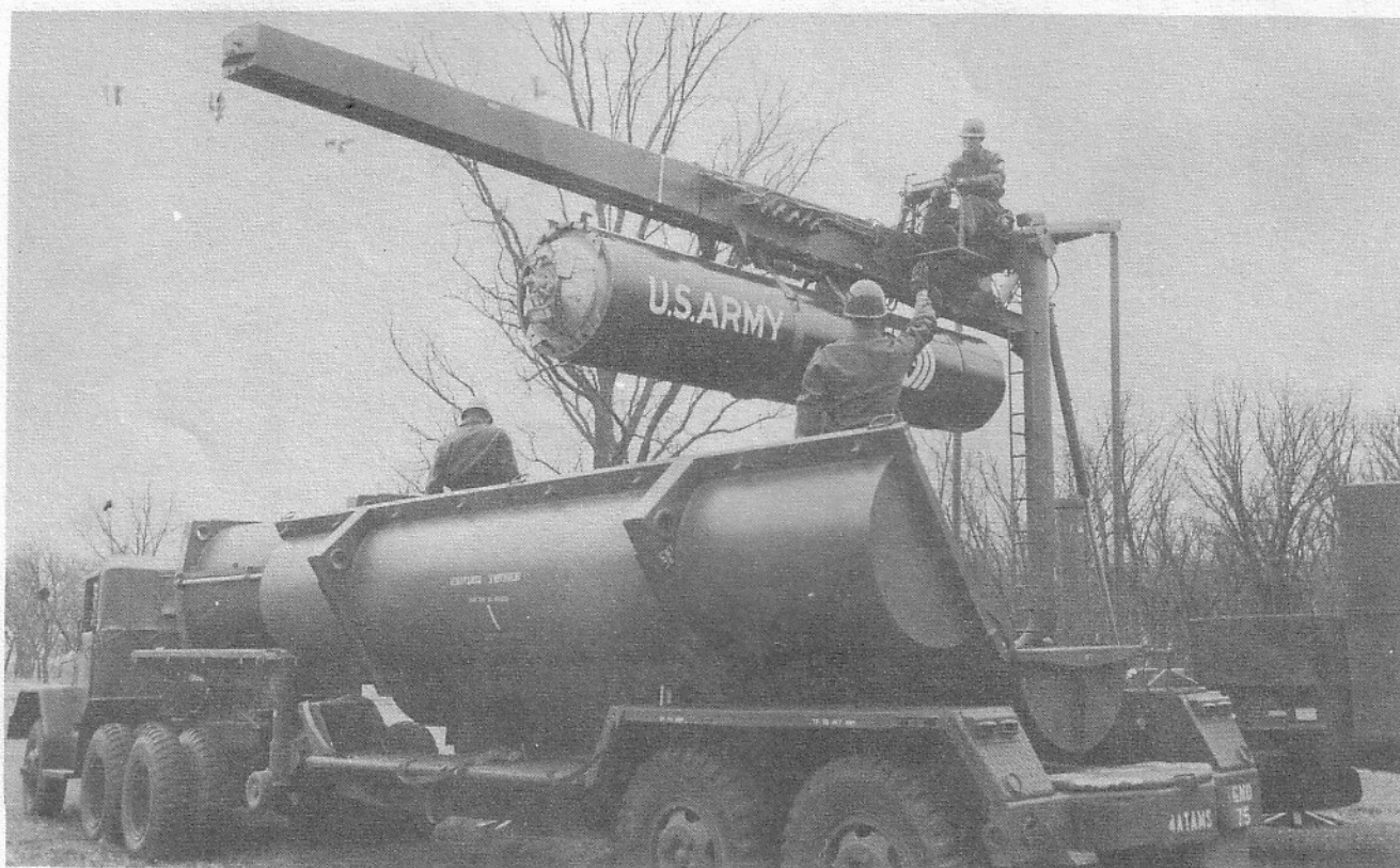
Figure 11. Positioning the rocket motor.
